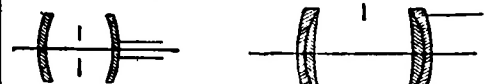
FIG. 25.—C. A. Steinheil's "Periskop." FIG. 26.—A. Steinheil's "Aplanat." by C. C. Harrison's "Globe Lens" (1862), angle 75^\circ , composed of a symmetrical pair of deep compound menisci, the exterior surfaces forming part of a sphere. Though defective and slow it was popular for a time. C. A. Steinheil's "Periskop" (1865, f/13.5 , angle 90^\circ ), was a symmetrical doublet formed of two plain crown menisci with central diaphragm (fig. 25). It gave a larger field than the "Globe," the lenses being closer together. Being nonachromatic it had to be adjusted for chemical focus. It was quite free from distortion, with a very flat field, and both nodal points together. It is considered the best possible combination of two plain lenses, and is still used in some of the cheaper hand cameras with fixed focus, the difference of the chemical and visual foci being allowed for in the camera or by adjustable lens mounts. G. Rodenstock's "Bistigmata" are of this class. J. Zentmayer made a similar unsymmetrical lens. In A. Steinheil's "Aplanat" (1866) the same principle was carried out with achromatized lenses, and a great
